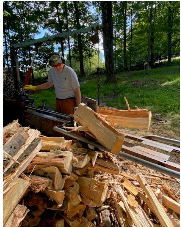
Ed Johnson cutting 32" black birch sticks for his sugarhouse on a splitter he made right there on his farm. The split wood goes on a pallet, and he burns 15 – 16 pallets each sugaring season. Each pallet is roughly \frac{1}{4} of a cord of wood.
